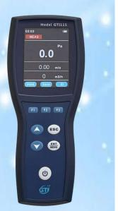
GTI 115 It is a high-precision differential pressure tester for non-corrosive gases. It can be connected to a Pitot tube to measure wind speed and air volume. With data storage function and export function, it is more convenient for users to use.
